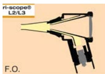
Fiber optics with 21.5-V/3.5-V XL xenon or 3.5-V LED illumination ensure an unhindered, glare-free view.
