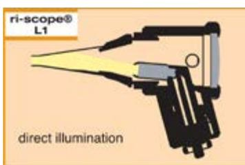
Reflection-reduced, cost-effective direct illumination with 2.5-V HL halogen or 3.5-V xenon lamps.
